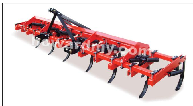
The HOWARD TINE TILLER is a simple strong unit suitable for secondary cultivation in good or marginal conditions. The tine, which is spring loaded, each with two springs, will swing back under a breakway pressure of approximately 308 lbs. and pass over any obstructions; returning to work once past the onbstruction without affecting the working depth of any of the other times.
