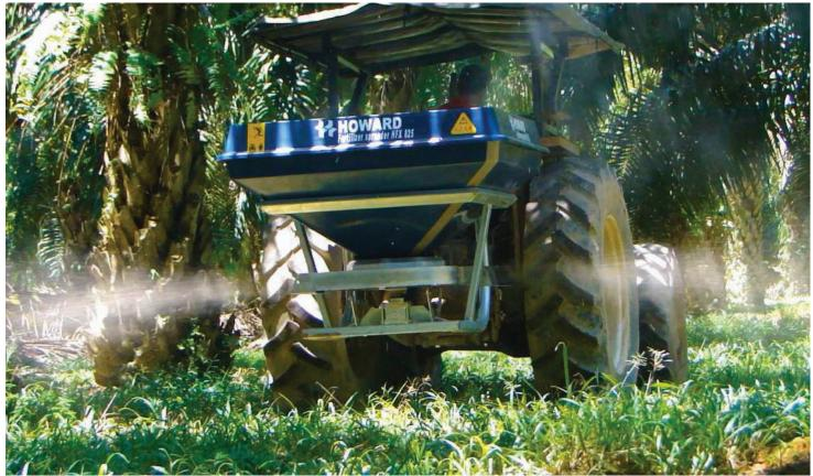
HOWARD HFX 825 is single disc spinner with stainless-steel chutes for band spreading up to 18m width. Glass-fibre hopper and adjustable chute deflectors for upwards and downwards direction of throw. Galvanized frame.
