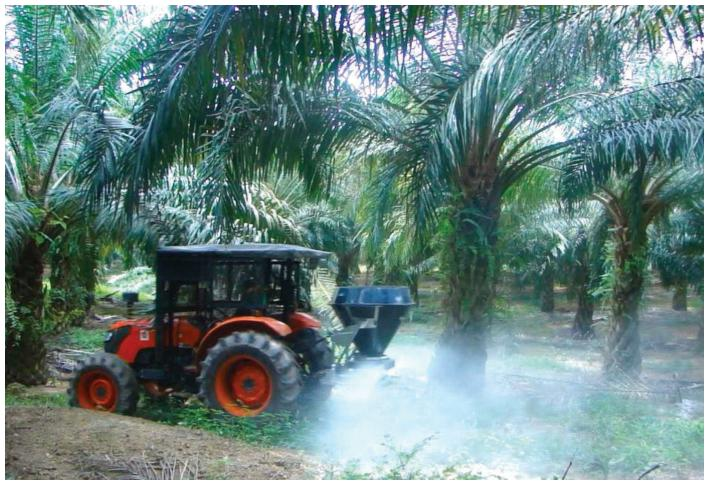
HOWARD HFX 525 is single disc spinner with stainless-steel chutes for band spreading up to 18m width. Glass-fibre hopper and adjustable chute deflectors for upwards and downwards direction of throw. Galvanized frame.
