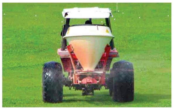
HFS 502 is a single-disc broadcaster, with stain-less steel agitator, spinner and throwers. Steep wall glass-fibre hopper with sturdy tube frame. Easy maintenance and service.
